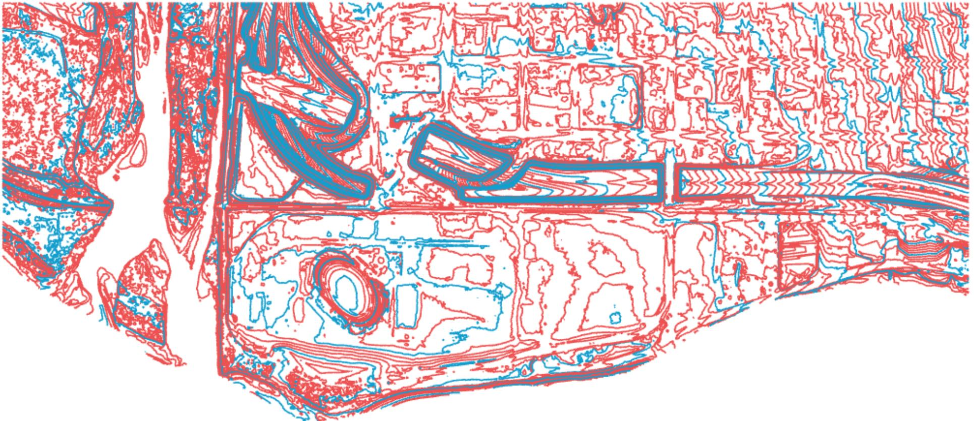
LIDAR contour lines are lines on a map that show points of equal elevation, generated from high-accuracy elevation data collected by LIDAR technology. LIDAR uses lasers to measure distances and create a detailed 3D point cloud of the ground, which is then used to generate these contour lines. The density of the lines indicates the steepness of the terrain: closely spaced lines show a steep slope, while widely spaced lines indicate a gentler slope.
