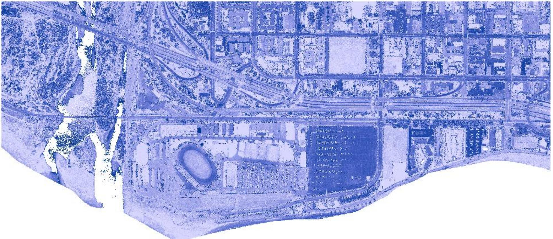
A LiDAR intensity image is a black-and-white image created from LiDAR data that represents the return strength of the laser pulse, similar to a grayscale photograph. It shows how much energy was reflected back to the sensor by each surface, with brighter areas indicating higher reflectivity and darker areas showing lower reflectivity. These images are useful for identifying features like roads, buildings, and vegetation, aiding in object classification and mapping.
