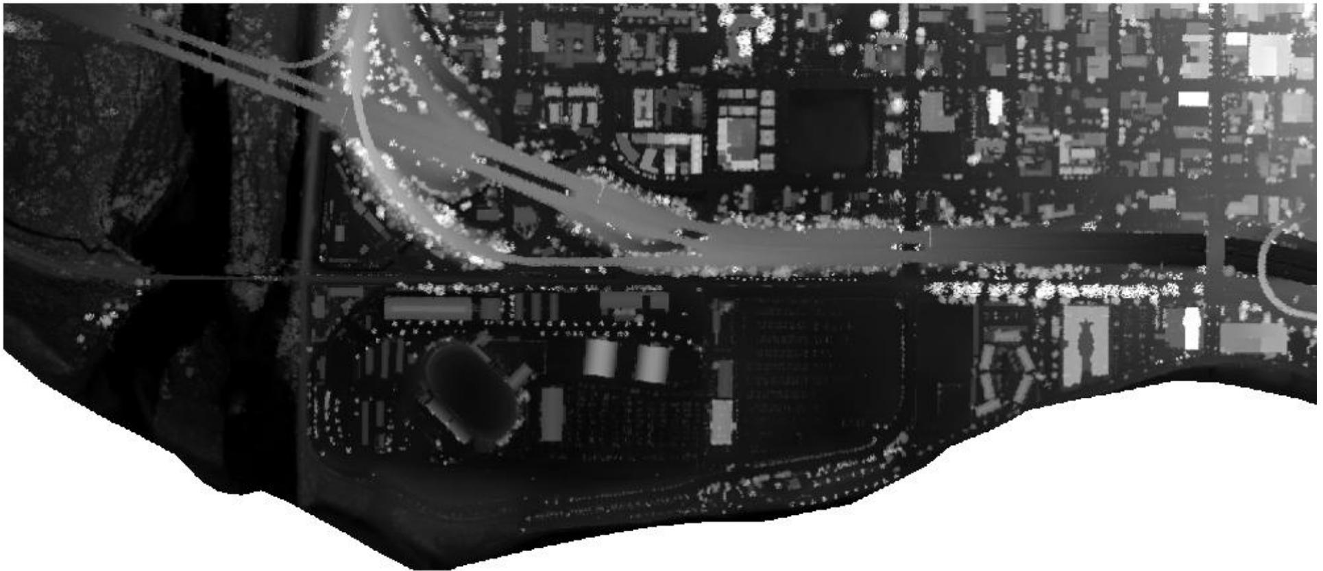
A [LiDAR](#) Digital Surface Model (DSM) is a 3D representation of the Earth's surface that includes the height of all objects on it, such as buildings, trees, and other man-made or natural features. LiDAR is a remote sensing method that uses laser pulses to measure distances, which are then used to create the DSM by capturing the elevation of the topmost surface, including all obstructions.
