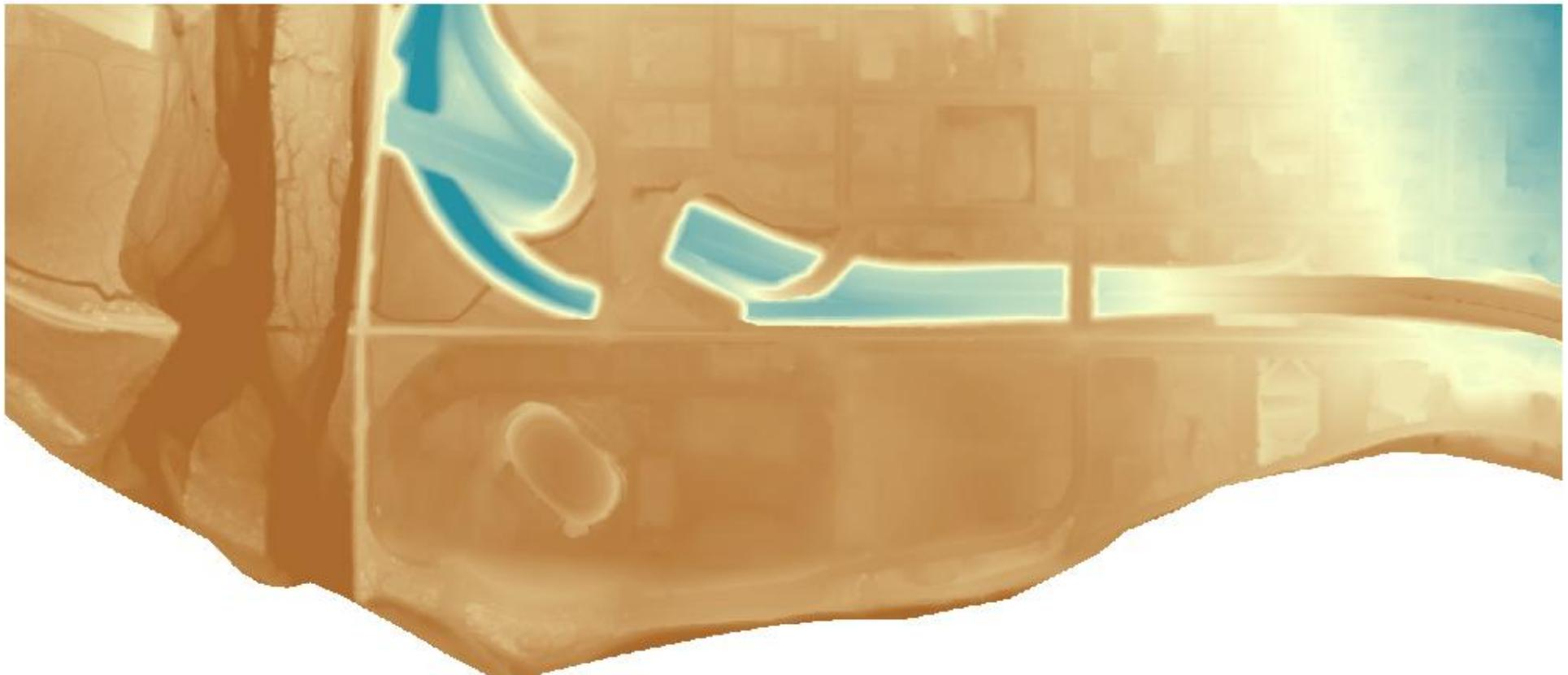
A [LiDAR bare earth DEM](#) is a high-resolution map of the Earth's surface created using LiDAR technology to show the ground elevation without any trees, buildings, or other structures. It is created by filtering out the "first returns" from laser pulses, which hit the top of objects, and instead using the last returns that reflect off the ground. This provides a true representation of the terrain itself.
