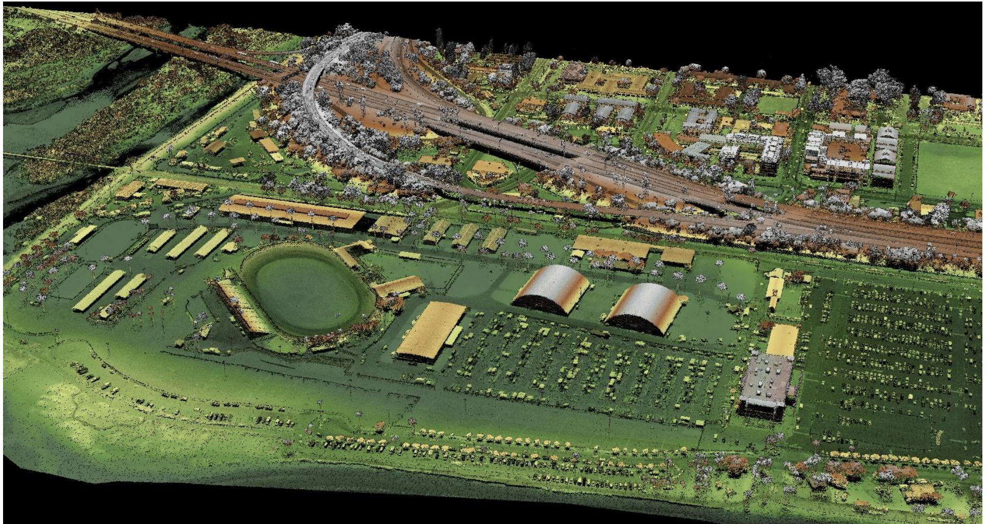
A LiDAR point cloud is a collection of 3D data points that represent an environment, created by a [LiDAR sensor](#) emitting laser pulses and measuring the time it takes for the light to reflect back. These points are used to build a detailed 3D model, and each point contains information such as its X, Y, and Z coordinates, as well as other attributes like intensity, color, and classification.
